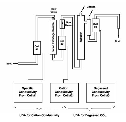
Figure 5-6 UDA for Cation and Degassed CO<sub>2</sub>
